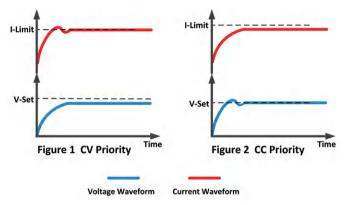
As shown in figure one, when the DUT requires reducing voltage overshoot during test, such as supplying power to a low-voltage processor or FPGA core, voltage priority mode should be selected to obtain fast and smooth rise voltage.
